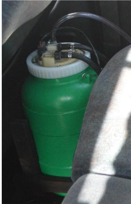
Fig. 2. A 12-liter tank for fuel
