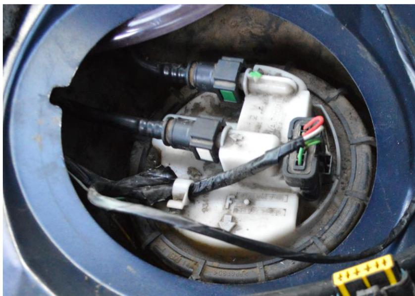
Fig. 1. In tank fuel pump
