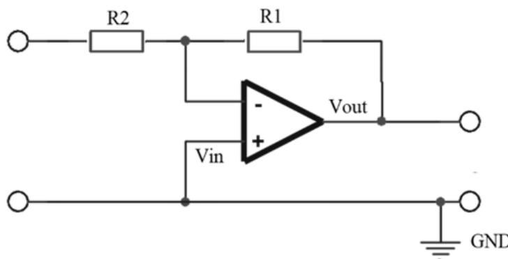
Fig. 1. Basic closed loop non-inverting operational amplifier circuit
