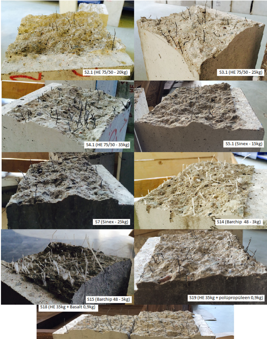
Figs 19-27. Failure modes of concretes reinforced with different fibres
