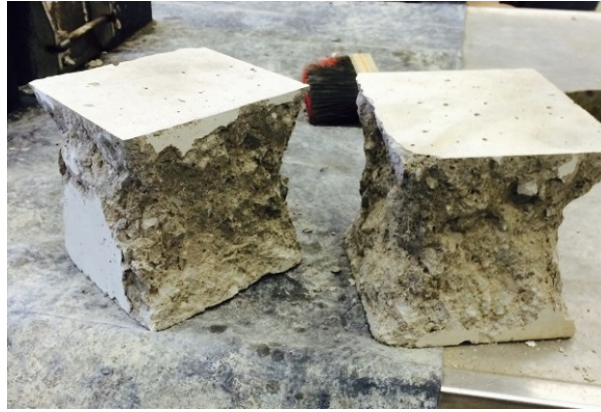
Fig. 14. The failure modes of compressive strength test specimens
